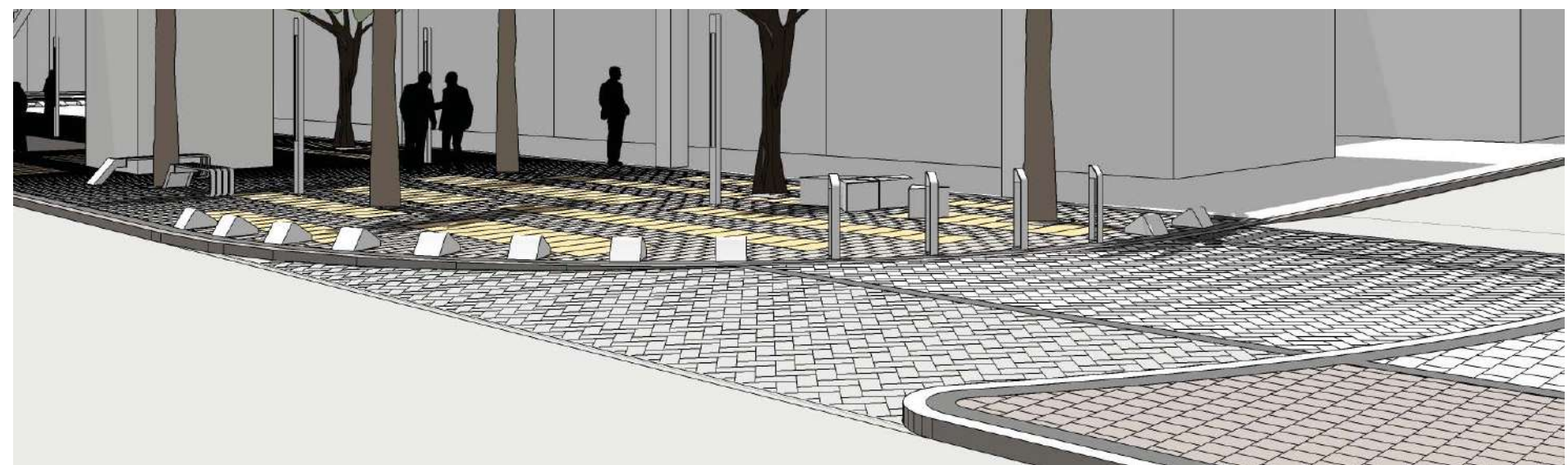
Figure 5.13 Application of raised table, including ramp 1:10 and bollards to restrict vehicular access onto walkway
