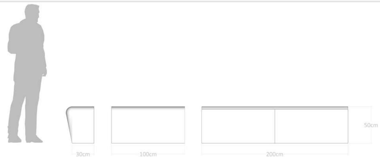
Figure 3.65 Raised planter - modular system with integrated seating
