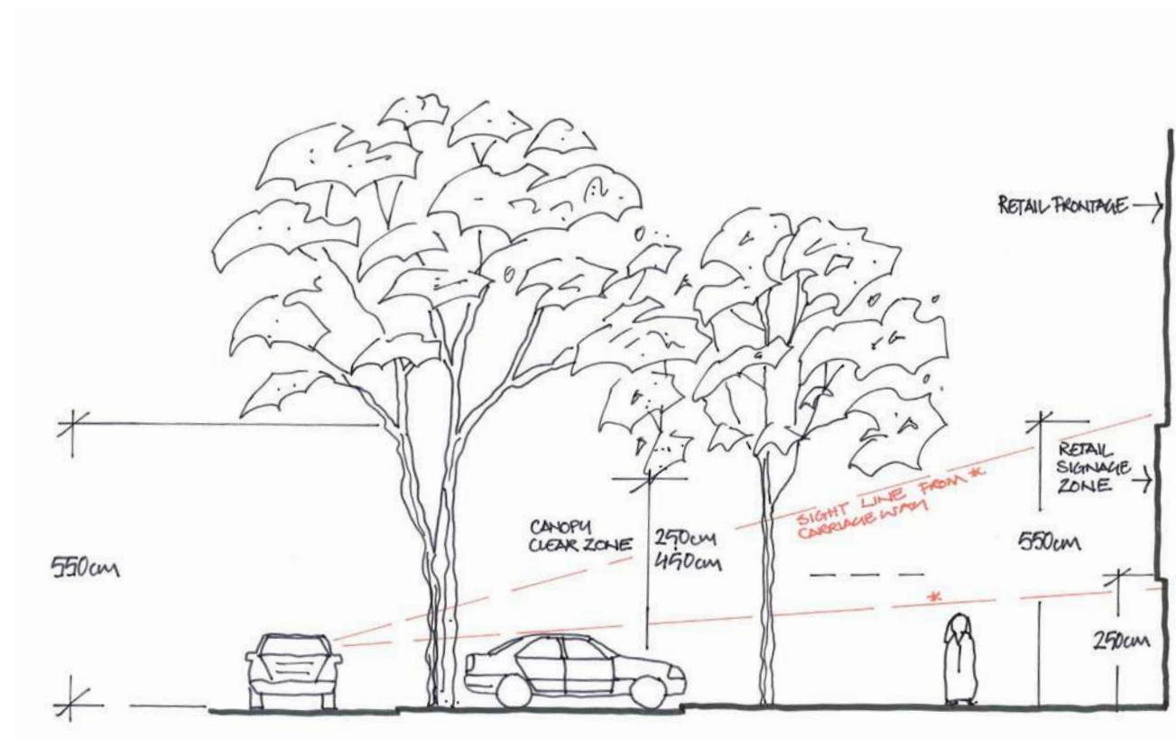
Figure 5.93 Sketch illustrating canopy clearance zones to pedestrian realm and carriageway
